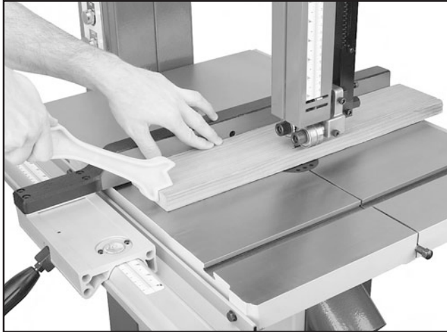
Figure 43. Ripping with a push stick.
